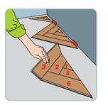
12. Once cut construct the triangles from the cut planks. Begin to install from the left hand side of the wall, a small amount of glue into the groove is recommended for some of the smaller pieces.
