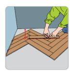
10a. Using a tape mark off positions to form a cut line across the run of flooring maintaining an equal distance to the starting wall.
