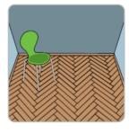
17. Once the flooring has been completed the spacers can be removed, using a scotia, beading or skirting the expansion gap can be covered to finish the project
