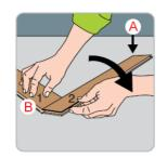
2. To connect plank No.2 (Type B) press the long side of the plank at an angle into the short side of the previous installed plank, folding the second panel to the floor will lock them together, checking that the grooves form a continues line
