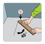
1. Select a wall to start your installation, and from the left hand corner place plank no.1 (Type A) with the longer male edge facing the wall to the left at an angle of 45°, ensure that the distance between the edge of plank No.1 and the wall is less than the distance of a full board.
